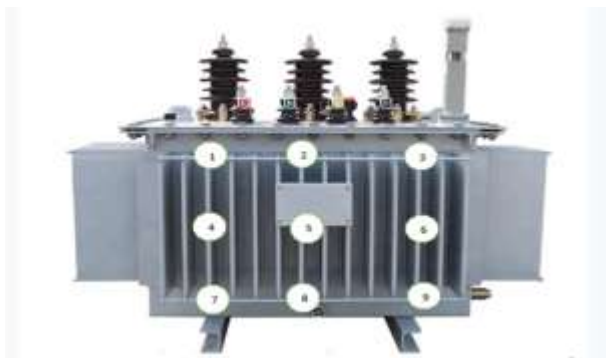
Figure 1. Points for measuring the level of vibration of the wall of the transformer tank.
