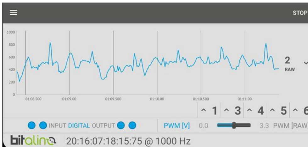
Figura 2. The result obtained from the ECG of the Bitalino device from the bioelectric activity of the heart
